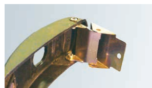
Composite material latch for wheel cover
