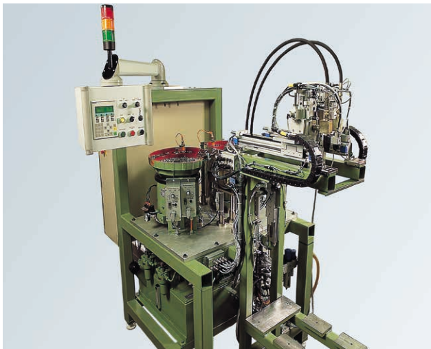
MIRS System to assemble vacuum pump
