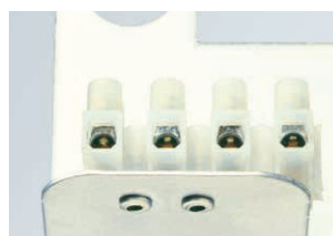
PVC connector block in air conditioning unit
