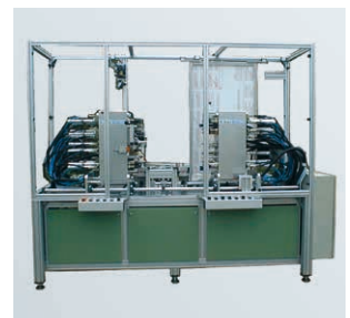
23 placing heads to assemble a computer chassis
